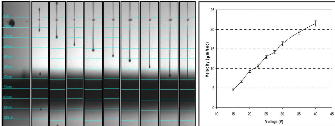
**Figure 3.** Adhesive drop images recorded at 30  $\mu\text{s}$  delay, showing distance traveled by cyanoacrylate drop with increasing voltage peaks (left to right). Graph shows the frontal velocity ( $\mu\text{m/s}$ ) vs. voltage (V) for the images (left to right).
