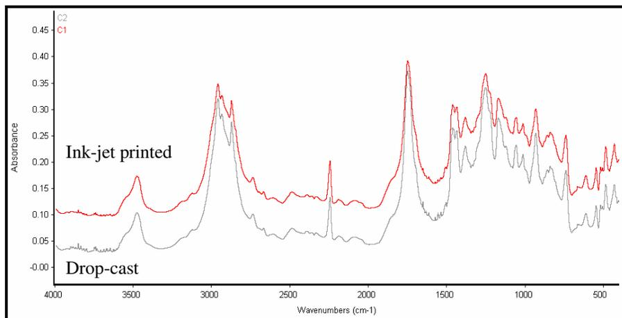
**Figure 6.** Fourier transform infrared absorption spectra overlay of ink-jet deposited and dropcast n-butyl cyanoacrylate adhesive.
