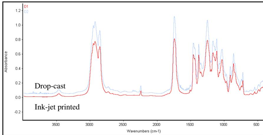
**Figure 7.** Fourier transform infrared absorption spectra overlay of ink-jet deposited and dropcast 2-octyl cyanoacrylate adhesive.
