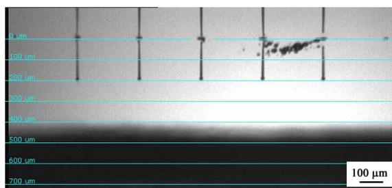
**Figure 2.** Optical micrograph of cyanoacrylate adhesive monomer release from five 21  $\mu\text{m}$  nozzles at 30  $\mu\text{s}$ .
