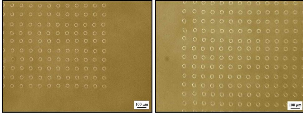
**Figure 5.** Optical micrograph of 2-octyl cyanoacrylate microarray patterns on 1% agarose gel.
