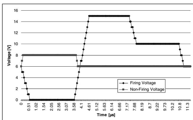
**Figure 1.** A sample voltage waveform used for jetting adhesives
