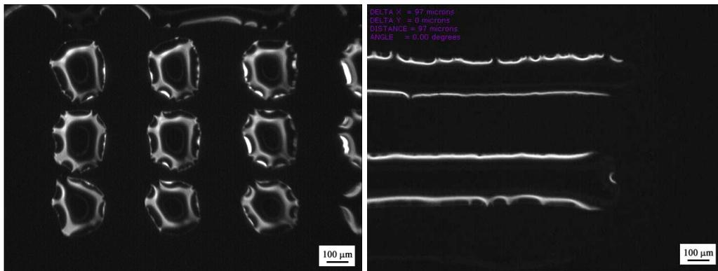
**Figure 4.** Optical micrograph of n-butyl cyanoacrylate patterns on silicon substrates.
