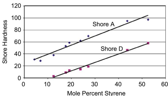
Fig. 8. Plot of mole percent styrene in SIBS versus shore hardness (courtesy of Yonghua Zhou and John B. Martin (Innovia LLC, Miami, FL)).
