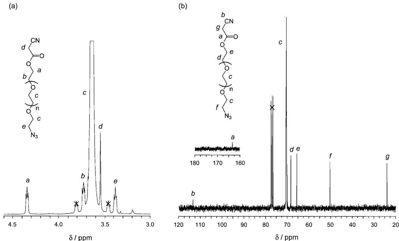
**Figure 2.** 400 MHz <sup>1</sup>H (a) and 75 MHz <sup>13</sup>C (b) NMR spectra in CDCl<sub>3</sub> of the azidopoly(ethylene glycol) cyanoacetate (N<sub>3</sub>PEG<sub>47</sub>CA, **7a**) synthesized following Path A (see Scheme 2).
