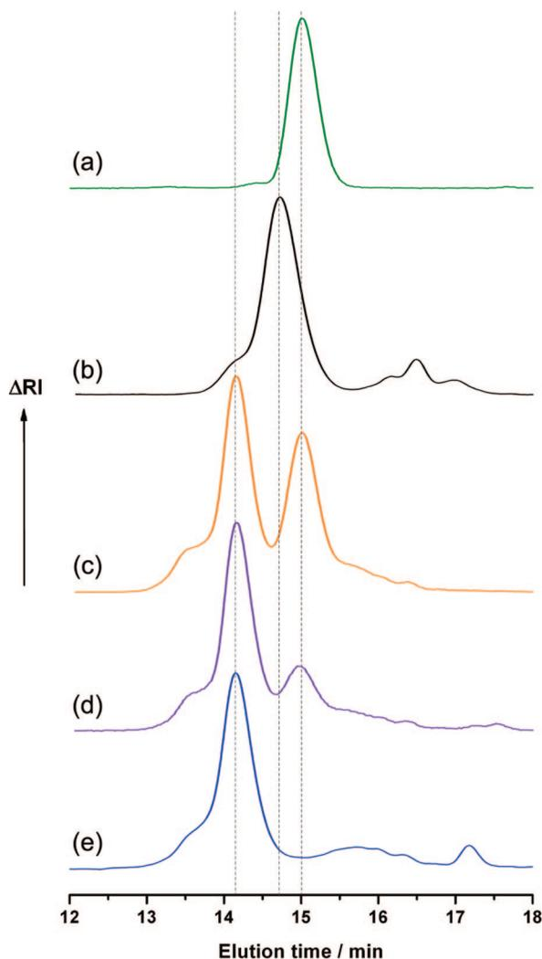
**Figure 8.** Size exclusion chromatography analysis of alkyne-PEG<sub>43</sub> (a), poly[(hexadecyl cyanoacrylate)-*co*-azidopoly(ethylene glycol) cyanoacrylate] P(HDCA-*co*-N<sub>3</sub>PEG<sub>70</sub>CA) copolymer before (b) and after click reaction with alkyne-PEG<sub>43</sub> in aqueous dispersed medium at various dialysis times (c–e).
