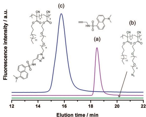
**Figure 6.** Size exclusion chromatography analysis with a fluorescence detector ( $\lambda_{\text{ex.}} = 340 \text{ nm}$ ;  $\lambda_{\text{em.}} = 520 \text{ nm}$ ) of alkyne-dansyl (a), poly[(hexadecyl cyanoacrylate)-*co*-azidopoly(ethylene glycol) cyanoacrylate] (P(HDCA-*co*-N<sub>3</sub>PEG<sub>47</sub>CA)) copolymer before (b) and after click reaction with alkyne-dansyl in *N,N*-dimethylformamide followed by dialysis (c).
