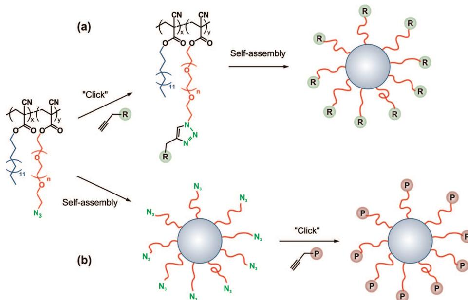
**Figure 1.** General approach to prepare functionalized poly(alkyl cyanoacrylate) nanoparticles: click reaction on the poly[(hexadecyl cyanoacrylate)-*co*-methoxypoly(ethylene glycol) cyanoacrylate] (P(HDCA-*co*-N<sub>3</sub>PEGCA)) copolymer followed by self-assembly in aqueous solution (a) or click reaction at the surface of preformed P(HDCA-*co*-N<sub>3</sub>PEGCA) nanoparticles (b).
