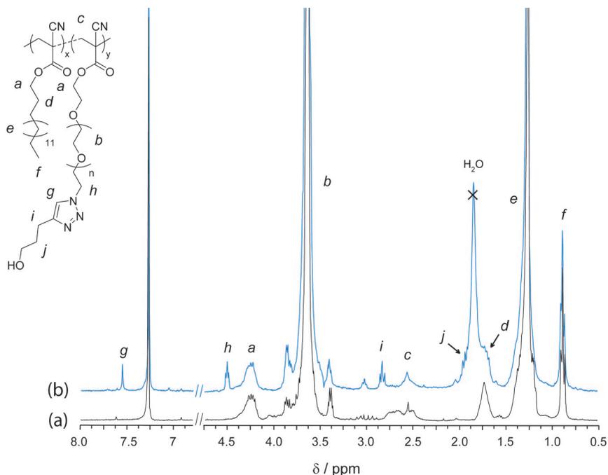
**Figure 5.** 300 MHz <sup>1</sup>H NMR spectrum in CDCl<sub>3</sub> of the poly[(hexadecyl cyanoacrylate)-*co*-azidopoly(ethylene glycol) cyanoacrylate] (P(HDCA-*co*-N<sub>3</sub>PEG<sub>70</sub>CA)) copolymer before (a) and after (b) click reaction with 4-pentyn-1-ol in *N,N*-dimethylformamide.
