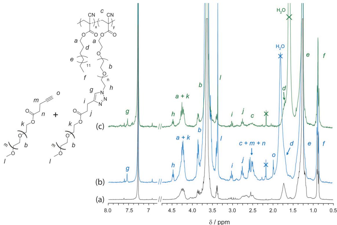
**Figure 7.** 300 MHz <sup>1</sup>H NMR spectrum in CDCl<sub>3</sub> of the poly[(hexadecyl cyanoacrylate)-*co*-azidopoly(ethylene glycol) cyanoacrylate] (P(HDCA-*co*-N<sub>3</sub>PEG<sub>70</sub>CA)) nanoparticles before (a), after the click reaction with alkyne-PEG<sub>43</sub> in aqueous dispersed medium (b), and after dialysis (c).
