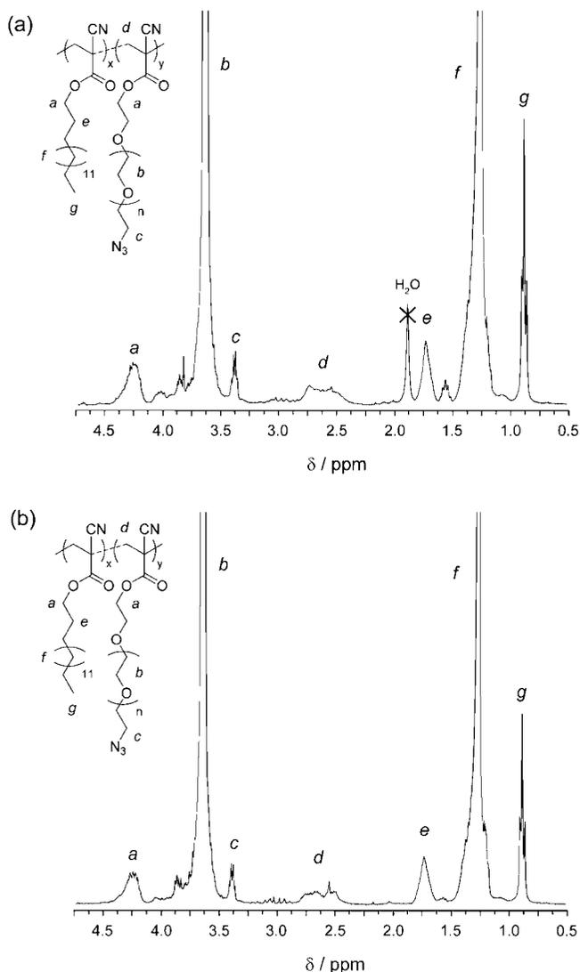
**Figure 3.** 300 MHz  $^1\text{H}$  NMR spectrum in  $\text{CDCl}_3$  of the poly[(hexadecyl cyanoacrylate)-*co*-azidopoly(ethylene glycol) cyanoacrylate] (P(HDCA-*co*- $\text{N}_3\text{PEG}_n\text{CA}$ )) copolymer;  $n = 47$  (a) and  $70$  (b).
